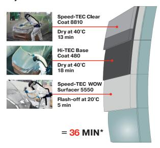
\*36 minutes repair time is based on new replacement parts (e-coat) wet-on-wet, no bare metal areas (no wipes). Includes application, flash-off and drying times.
